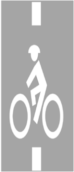
Figure 1-34: Bike symbol for loop detection placement
